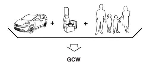
**GCW (Gross Combination Weight)** is the weight of the loaded vehicle (GVW) plus the weight of the fully loaded trailer.
